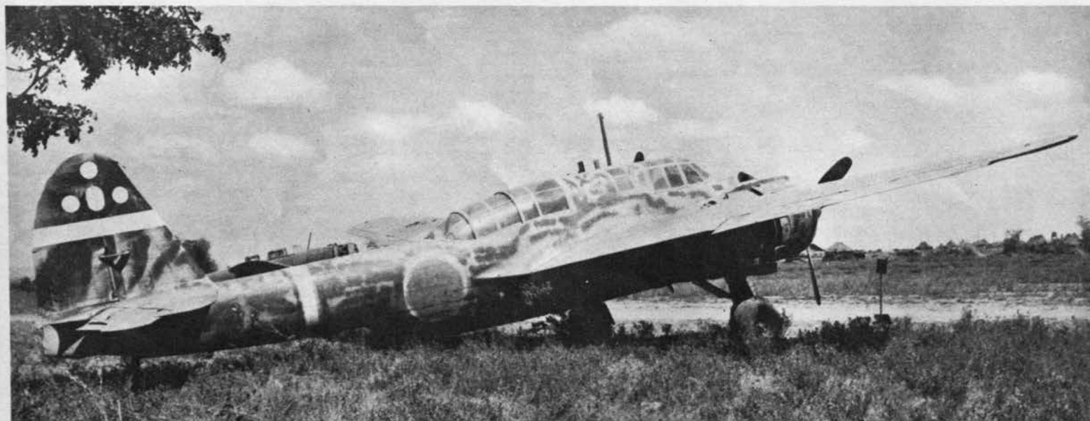
LILY Although still classified as a light bomber, Lily is likely to become more important as a divebomber. This is indicated by dive brakes found in the latest version. Lily's bulging belly
